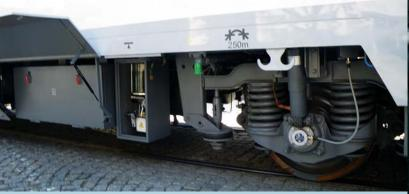
Wheel flange lubrication OK-02 is designed for locomotives which are equipped with their own source and distribution of pressure air. The system works on the principle of applying lubricant mixture to the contact area of locomotives wheel flanges with rails by means of pressure air.
